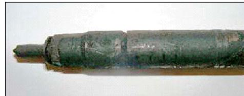
This injector has been seating correctly; the seat and copper washers have prevented any blow-by.
